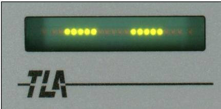
This has proven to be very effective in the final tuning of difficult tones. With this high-precision display, deviations less than 1/100 Hertz can still be registered.
